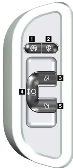
Figure 11: Gantry Control Panel
